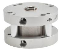
NITRA pneumatic cylinder, compact, 2-1/2in bore, 3/4in rod diameter, 1in stroke, double acting, counter-bored holes mount.
