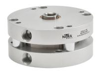
NITRA pneumatic cylinder, compact, 2-1/2in bore, 3/4in rod diameter, 1/2in stroke, double acting, counter-bored holes mount.
