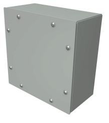
Hammond enclosure, NEMA 3/4/12, 8 x 8 x 4in (HxWxD), wall mount, carbon steel, ANSI 61 gray, powder coat finish, screw cover.
