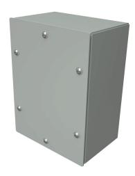
Hammond enclosure, NEMA 3/4/12, 8 x 6 x 4in (HxWxD), wall mount, carbon steel, ANSI 61 gray, powder coat finish, screw cover.
