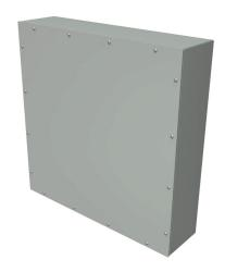
Hammond enclosure, NEMA 3/4/12, 24 x 24 x 6in (HxWxD), wall mount, carbon steel, ANSI 61 gray, powder coat finish, screw cover.
