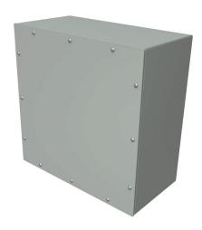
Hammond enclosure, NEMA 3/4/12, 16 x 16 x 8in (HxWxD), wall mount, carbon steel, ANSI 61 gray, powder coat finish, screw cover.
