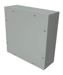
Hammond enclosure, NEMA 3/4/12, 12 x 12 x 4in (HxWxD), wall mount, carbon steel, ANSI 61 gray, powder coat finish, screw cover.
