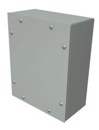
Hammond enclosure, NEMA 3/4/12, 10 x 8 x 4in (HxWxD), wall mount, carbon steel, ANSI 61 gray, powder coat finish, screw cover.
