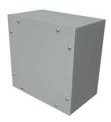
Hammond enclosure, NEMA 3/4/12, 10 x 10 x 6in (HxWxD), wall mount, carbon steel, ANSI 61 gray, powder coat finish, screw cover.
