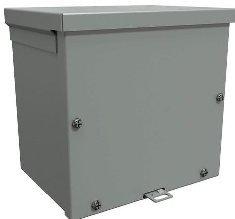
Hammond enclosure, NEMA 3R, 8 x 8 x 6in (HxWxD), wall mount, with knockouts, galvanized steel, ANSI 61 gray, powder coat finish, screw cover, padlock hasp and staple.
