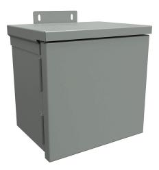
Hammond enclosure, NEMA 3R, 8 x 8 x 6in (HxWxD), wall mount, with knockouts, galvanized steel, ANSI 61 gray, powder coat finish, single-door, quick-release latch, padlock hasp and staple.
