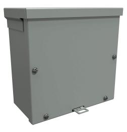
Hammond enclosure, NEMA 3R, 8 x 8 x 4in (HxWxD), wall mount, galvanized steel, ANSI 61 gray, powder coat finish, screw cover, padlock hasp and staple.
