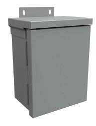
Hammond enclosure, NEMA 3R, 8 x 6 x 4in (HxWxD), wall mount, with knockouts, galvanized steel, ANSI 61 gray, powder coat finish, single-door, quick-release latch, padlock hasp and staple.
