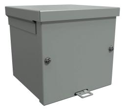
Hammond enclosure, NEMA 3R, 6 x 6 x 6 in (HxWxD), wall mount, with knockouts, galvanized steel, ANSI 61 gray, powder coat finish, screw cover, padlock hasp and staple.
