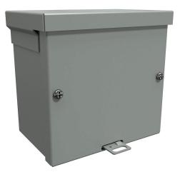
Hammond enclosure, NEMA 3R, 6 x 6 x 4in (HxWxD), wall mount, galvanized steel, ANSI 61 gray, powder coat finish, screw cover, padlock hasp and staple.
