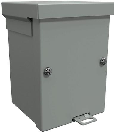
Hammond enclosure, NEMA 3R, 6 x 4 x 4in (HxWxD), wall mount, with knockouts, galvanized steel, ANSI 61 gray, powder coat finish, screw cover, padlock hasp and staple.
