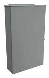
Hammond enclosure, NEMA 3R,  $60 \times 36 \times 12$ in (HxWxD), wall mount, galvanized steel, ANSI 61 gray, powder coat finish, hinged screw cover, padlock hasp and staple.
