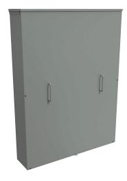
Hammond enclosure, NEMA 3R, 48 x 36 x 8in (HxWxD), wall mount, with knockouts, galvanized steel, ANSI 61 gray, powder coat finish, screw cover with handles, padlock hasp and staple.
