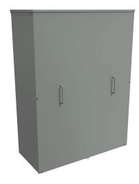
Hammond enclosure, NEMA 3R, 48 x 36 x 16in (HxWxD), wall mount, with knockouts, galvanized steel, ANSI 61 gray, powder coat finish, screw cover with handles, padlock hasp and staple.
