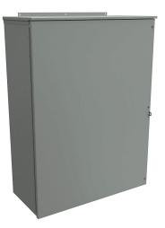
Hammond enclosure, NEMA 3R, 48 x 36 x 16in (HxWxD), wall mount, galvanized steel, ANSI 61 gray, powder coat finish, hinged screw cover, padlock hasp and staple.
