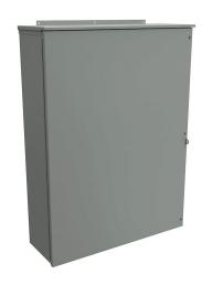
Hammond enclosure, NEMA 3R,  $48 \times 36 \times 12$ in (HxWxD), wall mount, galvanized steel, ANSI 61 gray, powder coat finish, hinged screw cover, padlock hasp and staple.
