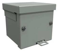
Hammond enclosure, NEMA 3R, 4 x 4 x 4 in (HxWxD), wall mount, with knockouts, galvanized steel, ANSI 61 gray, powder coat finish, screw cover, padlock hasp and staple.
