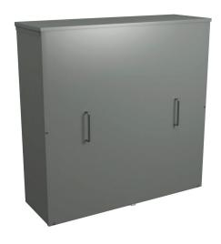
Hammond enclosure, NEMA 3R,  $36 \times 36 \times 12$ in (HxWxD), wall mount, galvanized steel, powder coat finish, screw cover, padlock hasp and staple.
