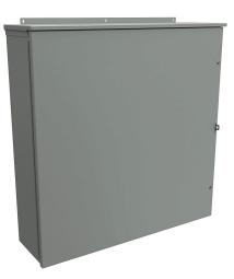
Hammond enclosure, NEMA 3R, 36 x 36 x 10in (HxWxD), wall mount, galvanized steel, ANSI 61 gray, powder coat finish, hinged screw cover, padlock hasp and staple.
