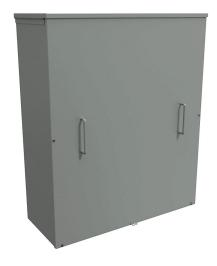
Hammond enclosure, NEMA 3R, 36 x 30 x 12in (HxWxD), wall mount, with knockouts, galvanized steel, ANSI 61 gray, powder coat finish, screw cover with handles, padlock hasp and staple.
