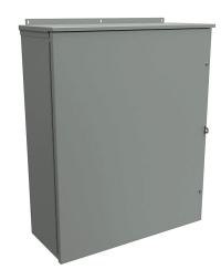
Hammond enclosure, NEMA 3R, 36 x 30 x 12in (HxWxD), wall mount, galvanized steel, ANSI 61 gray, powder coat finish, hinged screw cover, padlock hasp and staple.
