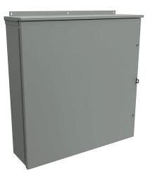
Hammond enclosure, NEMA 3R, 30 x 30 x 8in (HxWxD), wall mount, galvanized steel, ANSI 61 gray, powder coat finish, hinged screw cover, padlock hasp and staple.
