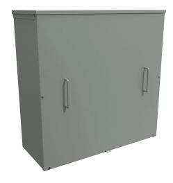
Hammond enclosure, NEMA 3R, 30 x 30 x 12in (HxWxD), wall mount, with knockouts, galvanized steel, ANSI 61 gray, powder coat finish, screw cover with handles, padlock hasp and staple.
