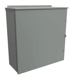
Hammond enclosure, NEMA 3R,  $30 \times 30 \times 12$ in (HxWxD), wall mount, galvanized steel, ANSI 61 gray, powder coat finish, hinged screw cover, padlock hasp and staple.
