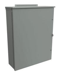
Hammond enclosure, NEMA 3R, 30 x 24 x 8in (HxWxD), wall mount, galvanized steel, ANSI 61 gray, powder coat finish, hinged screw cover, padlock hasp and staple.
