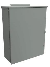
Hammond enclosure, NEMA 3R, 30 x 24 x 10in (HxWxD), wall mount, galvanized steel, ANSI 61 gray, powder coat finish, hinged screw cover, padlock hasp and staple.
