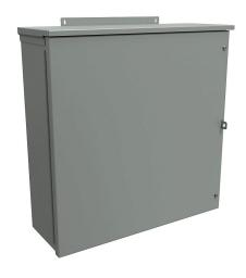
Hammond enclosure, NEMA 3R, 24 x 24 x 8in (HxWxD), wall mount, galvanized steel, ANSI 61 gray, powder coat finish, hinged screw cover, padlock hasp and staple.
