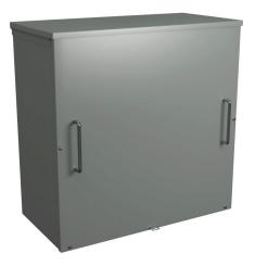
Hammond enclosure, NEMA 3R, 24 x 24 x 12in (HxWxD), wall mount, galvanized steel, powder coat finish, screw cover, padlock hasp and staple.
