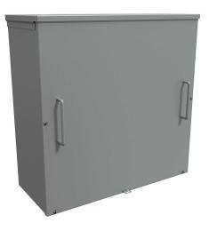
Hammond enclosure, NEMA 3R, 24 x 24 x 10in (HxWxD), wall mount, with knockouts, galvanized steel, ANSI 61 gray, powder coat finish, screw cover with handles, padlock hasp and staple.
