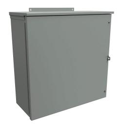
Hammond enclosure, NEMA 3R, 24 x 24 x 10in (HxWxD), wall mount, galvanized steel, ANSI 61 gray, powder coat finish, hinged screw cover, padlock hasp and staple.
