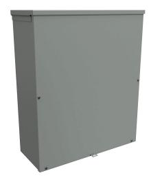
Hammond enclosure, NEMA 3R, 24 x 20 x 8in (HxWxD), wall mount, with knockouts, galvanized steel, ANSI 61 gray, powder coat finish, screw cover, padlock hasp and staple.
