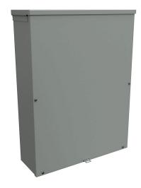
Hammond enclosure, NEMA 3R, 24 x 18 x 6in (HxWxD), wall mount, with knockouts, galvanized steel, ANSI 61 gray, powder coat finish, screw cover, padlock hasp and staple.
