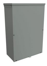
Hammond enclosure, NEMA 3R, 24 x 16 x 8in (HxWxD), wall mount, with knockouts, galvanized steel, ANSI 61 gray, powder coat finish, screw cover, padlock hasp and staple.
