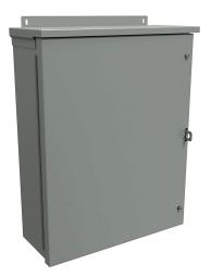
Hammond enclosure, NEMA 3R, 20 x 16 x 6in (HxWxD), wall mount, galvanized steel, ANSI 61 gray, powder coat finish, hinged screw cover, padlock hasp and staple.
