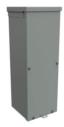
Hammond enclosure, NEMA 3R, 18 x 6 x 6in (HxWxD), wall mount, with knockouts, galvanized steel, ANSI 61 gray, powder coat finish, screw cover, padlock hasp and staple.
