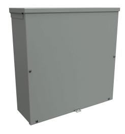
Hammond enclosure, NEMA 3R, 18 x 18 x 6in (HxWxD), wall mount, with knockouts, galvanized steel, ANSI 61 gray, powder coat finish, screw cover, padlock hasp and staple.
