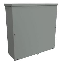
Hammond enclosure, NEMA 3R, 18 x 18 x 6in (HxWxD), wall mount, galvanized steel, ANSI 61 gray, powder coat finish, screw cover, padlock hasp and staple.
