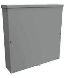
Hammond enclosure, NEMA 3R, 18 x 18 x 4in (HxWxD), wall mount, with knockouts, galvanized steel, ANSI 61 gray, powder coat finish, screw cover, padlock hasp and staple.
