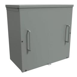
Hammond enclosure, NEMA 3R, 18 x 18 x 10in (HxWxD), wall mount, with knockouts, galvanized steel, ANSI 61 gray, powder coat finish, screw cover with handles, padlock hasp and staple.
