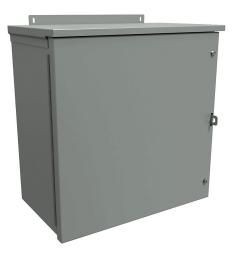
Hammond enclosure, NEMA 3R, 18 x 18 x 10in (HxWxD), wall mount, galvanized steel, ANSI 61 gray, powder coat finish, hinged screw cover, padlock hasp and staple.
