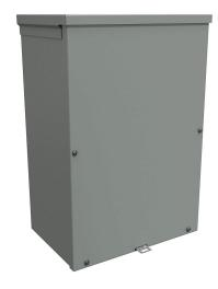
Hammond enclosure, NEMA 3R, 18 x 12 x 8in (HxWxD), wall mount, with knockouts, galvanized steel, ANSI 61 gray, powder coat finish, screw cover, padlock hasp and staple.
