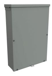
Hammond enclosure, NEMA 3R, 18 x 12 x 4in (HxWxD), wall mount, with knockouts, galvanized steel, ANSI 61 gray, powder coat finish, screw cover, padlock hasp and staple.
