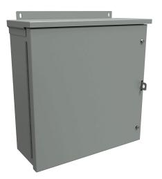
Hammond enclosure, NEMA 3R, 16 x 16 x 6in (HxWxD), wall mount, galvanized steel, ANSI 61 gray, powder coat finish, hinged screw cover, padlock hasp and staple.
