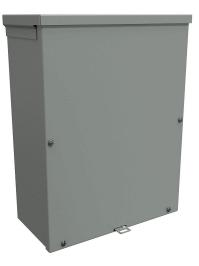
Hammond enclosure, NEMA 3R, 16 x 12 x 6in (HxWxD), wall mount, with knockouts, galvanized steel, ANSI 61 gray, powder coat finish, screw cover, padlock hasp and staple.
