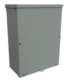
Hammond enclosure, NEMA 3R, 16 x 12 x 6in (HxWxD), wall mount, galvanized steel, ANSI 61 gray, powder coat finish, screw cover, padlock hasp and staple.
